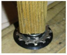
At this point all you need to do is put the two machined plates together, screw in the three screws and then put the pulley back on the linkage plate. Remember that the side with the three screws will face towards the frame.
