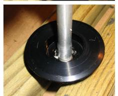
With both the bearings removed, it's now time to remove the axle that was inside the larger of these bearings. You can accomplish this by hammering it out with something like the socket wrench extender I used to get the smaller bearing out in the previous step.
