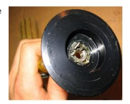
Here is a picture showing the smaller bearing still in the pulley. It also shows the metal wall I spoke of earlier that separates the bearings and the accidental damage I did to it while hammering.
