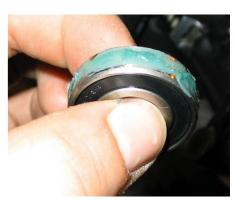
With the bearing greased up, insert it into the cup and then using a hammer and dowel, tap it in. Make sure that you do not damage the rubber seal of the bearing while you do this.
