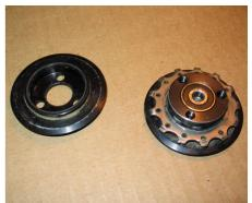
Now that you have the machined pulley sides apart, take a look at the piece that holds the bearings. There will be two bearings, one large with a metal axle insert and one small bearing. These two bearings are separated by a metal wall so you cannot simply hammer the smaller one directly against the larger bearing and make it pop out.
