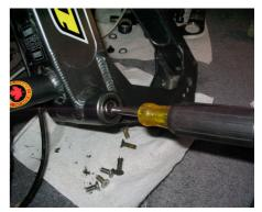
Below is a picture of the frame with one of the bearings removed. Notice that there is a bevel that keeps the bearings from moving too deep into the tube of the pivot.
