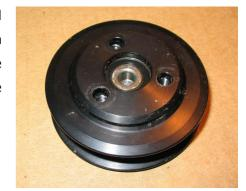
Using your fingers, pull the two sides apart. If it is difficult to do, try spraying it with WD-40. Now is probably a good time to clean out all that gunk in there. If the cog is really worn, you might want to replace that too. As mentioned earlier, it should just be a cog out of a standard cassette.
