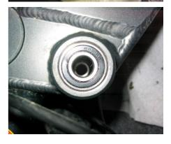
You can see in this picture that I hammered the axle through without a screw. I was able to avoid mashing the threads by putting a socket atop of the cone in a manner that did not mash the threads. But if I were to do it again, I would have threaded a screw in.
