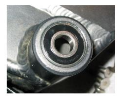
Now it is time to hammer in the axle. The best way to do this is to grab the link plate that does not have the pulley on it, put a little grease in the divet the axle cone goes into, then bolt the unit onto the axle. Afterwards, put on a washer and then lube up the entire length of the axle body (to allow it to slide in more easily and to stop squeaks). Once you have done all of this, tap in the axle until the linkage plate/washer is directly against the inner race of the bearing.
