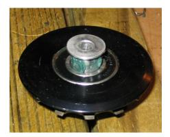
Once you have pushed it in a little ways, either use a dowel and hammer to hammer it into the bearing or use a vice to squeeze it in. Whichever way you choose to do this, make sure you don't harm the rubber seal of the bearing!
