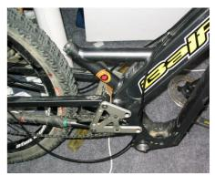
The first step to disassembling all this is to remove the rear triangle and the two screws that hold the pivot together. If you find you cannot unscrew both linkage plates, don't worry about it, only one needs to be unscrewed now.
