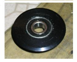
Remember that axle you hammered out earlier? Well grease it up and push it into the inner race of the bearing you just hammered in!
