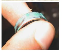
With the bearing greased up, use a hammer and dowel or a vice to squeeze it back into the cup it sits in. As with the larger bearing, make sure you don't harm the rubber seal!
