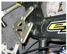
With the axle in, all you need to do for the other side (the side with the pulley) is to grease the divet in the linkage plate the axle is pushed into, add the washer, then screw the pivot bolt back in.
