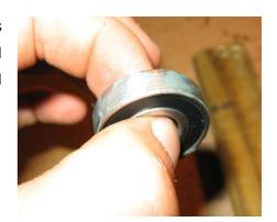
You will need to hammer (or push back into place with a vice) the big bearing back into the cup it sits in. Make sure that you do not damage the rubber seal of the bearing while doing this. If you have to hammer it back in, try using a dowel or piece of wood that covers the surface of the bearing. This will help distribute the force in addition to preventing you from mashing in the rubber seal.
