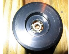
To remove the smaller bearing, find something about the size of the internal race. In my case I use a socket wrench extender.
