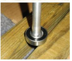
Notice the axle has a lip on it on one side. Make sure you are not trying to hammer it out the wrong.
